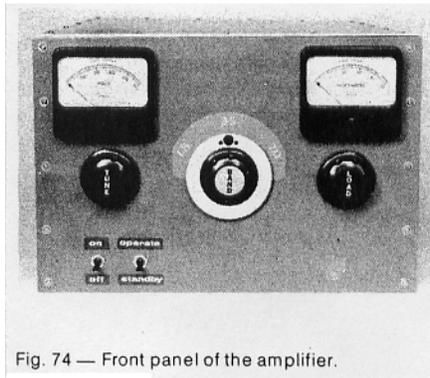
Fig. 74 — Front panel of the amplifier.
